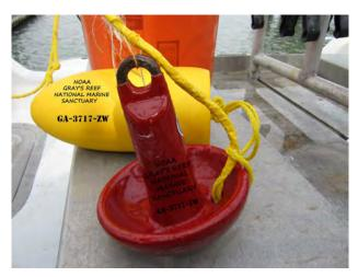
Gray's Reef vessel operators use an 8 pound mushroom anchor attached to a line and buoy float to mark the location of divers underwater. (Photo: Todd Recicar, Amy Rath)
