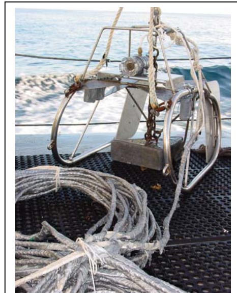
Figure 1. Camera and sled used to map benthic habitats within the vicinity of Gray's Reef National Marine Sanctuary. Photograph by Greg McFall.
