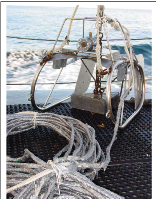
Figure 2. Seaview camera mounted on sled. Umbilical is in the foreground.
