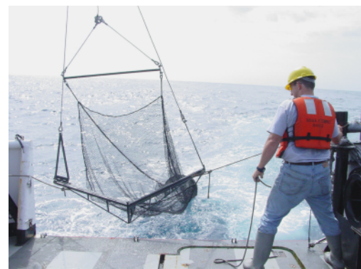
Figure 3. Deployment of the Issacs Kidd midwater trawl.
