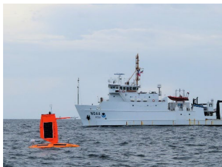
An uncrewed Saildrone collected ocean data for NOAA hurricane models while the Nancy Foster expedition conducted other research at Gray's Reef National Marine Sanctuary. Photo: Ben Prueitt/NOAA
